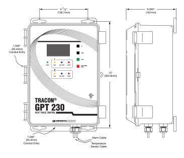
The GPT 230 Dual Channel Heat-Trace Control is a dual-point microprocessorbased heat-trace control thermostat. It is ideal for applications which require two independent heater-control Channels with Ground-Fault Equipment Protection (GFEP). Ideal uses include freeze protection, hot water temperature maintenance, grease line trace, tank heating, and other temperature monitoring and control applications.
