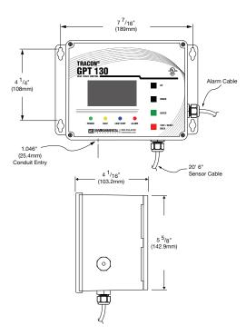
The GPT 130 Heat–Trace Control is a single–point microprocessor–based heat–trace control thermostat. It is ideal for applications which require Ground– Fault Equipment Protection (GFEP). Ideal uses include freeze protection, hot water temperature maintenance, grease line trace, tank heating, and other temperature monitoring and control applications.
