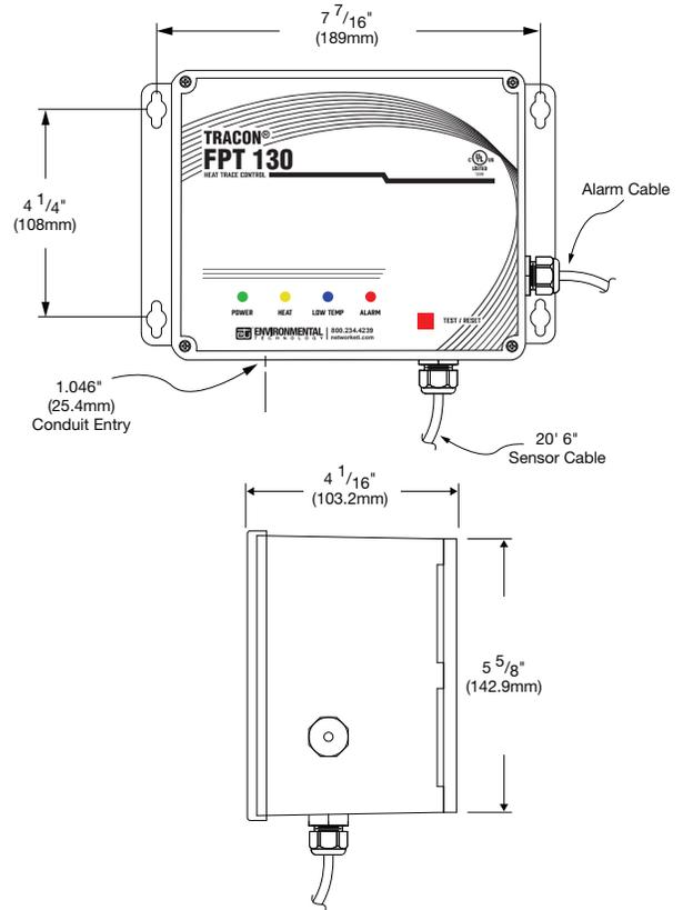
The FPT 130 Heat-Trace Control is a single-point microprocessor-based heat-trace control thermostat. It is ideal for applications which require Ground-Fault Equipment Protection (GFEP). Ideal uses include freeze protection, and other temperature monitoring and control applications.
