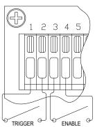
capability to trigger the system through telephone or computer control. Closure of the Trigger and Enable inputs will start one snow melting cycle, just as though the MANUAL ON button was pressed. Once the cycle is complete the sensor will revert to AUTOMATIC mode.
