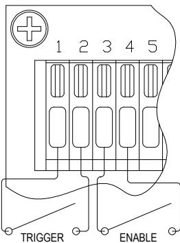
The Enable input is an optional connection point for a second "safety" contact set. If used, both contact sets must close to trigger the snow melt system. This can help eliminate inadvertent cycling of the system. If only one contact set is available the user may install a jumper wire across terminals 3 & 4. The user may also connect a simple toggle switch across the Enable input to allow manual enabling and disabling of the home automation interface.
