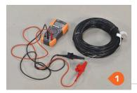
Before removing the cable from the spool, you need to conduct the resistance, continuity, insulation resistance tests. These first set f tests are required, please write the values obtained in the "Test Log" located on page 38.
