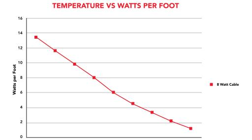
In Roof and Gutter De-icing applications where TRM SR-PL cables are surrounded by ice and snow, the cables will generate 12W per linear foot
