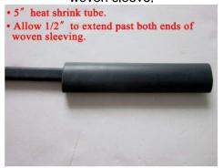
**7.** Apply heat evenly to the heat shrink tube until it shrinks around the cable.
