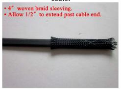
**6.** Slide the 125 mm (5") heat shrink tube over the woven braid sleeve, allowing 13mm (1/2") to extend past the each end of the woven sleeve.
