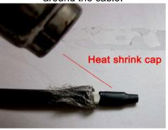
**4.** Pull the braid over the sealed end cap-and twist the braid ends together.
