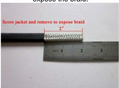
2. Push the braid back, and cut off the end 19 mm (3/4") of the base cable.
