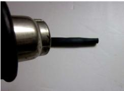
12. While the shrink tubing is still hot, gently squeeze the end of the shrink tube with pliers and hold until cool. The end must remain visibly sealed when the pliers are removed. If the tube does not remain sealed, then repeat steps 11 and 12.
