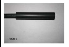
6.) **Figure 6**: Slide the heat shrink tubing (A) over the woven braid, allowing  $\frac{1}{2}$ " to extend past both ends of the braid.
