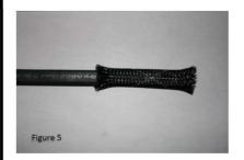
5.) Figure 5: Slide the woven braid sleeve (B) over the end of the cable, allowing  $\frac{1}{2}$ " to extend past the end of the cable.
