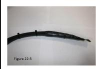
**22.) Figure 22-4/22-5**: Ensure the end of the heat shrink is completely sealed with adhesive.
