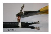
12.) Figure 12-1: Cut off the excess braid.
