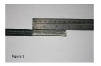
1.) **Figure 1**: Slice completely around the black outer jacket 2 ¾" from the cables end, being careful not to cut braid or inner jacket. Then, bend the cable where sliced to break jacket, and peel off.
