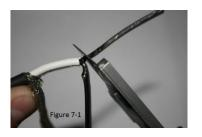
7.) **Figure 7-1**: using a utility knife, cut the matrix material around the base of each conductor. Be careful not to cut the conductor
