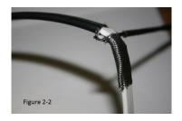
**2.) Figure 2-2**: Bend the cable and push the braid until there is enough room between the bottom of the cable and the braid to fit a screwdriver
