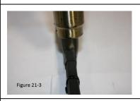
**21.) Figure 21-3**: When heating, work the heat gun side to side to ensure an even distribution of heat along the tube.
