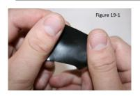
19.) **Figure 19-1**: Remove release paper from mastic strip (E) and stretch the width (1" side) of the mastic strip as shown. (Stretching the strips is necessary because the width cannot fully wrap around each of the heat shrink caps).
