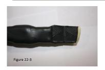
**22.)** Figure 22-2/22-3: If the width of the pliers isn't wide enough to pinch the entire tube, pinch a second time at the end of the cable.
