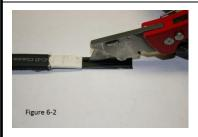
6.) Using either a pair of scissors (**Figure 6-1**) or a utility knife (**Figure 6-2**) make a cut through the centre matrix material 1 ¾", down to where the inner jacket begins (**Figure 6-3**).
