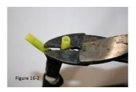
**16.) Figure 16-2**: Using a crimping tool, crimp each set of conductors together
