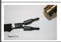
**17.)** Figure 17-2/17-3: Apply heat from the end of the cap evenly until it shrinks and adhesive flows out. If adhesive does not appear, additional heat is needed.
