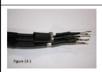
13.) **Figure 13-1**: Slide the black heat shrink tube (J) over uninsulated braid crimp (K).
